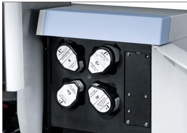
Figure 4. Four-lamp mount for maximum flexibility.
