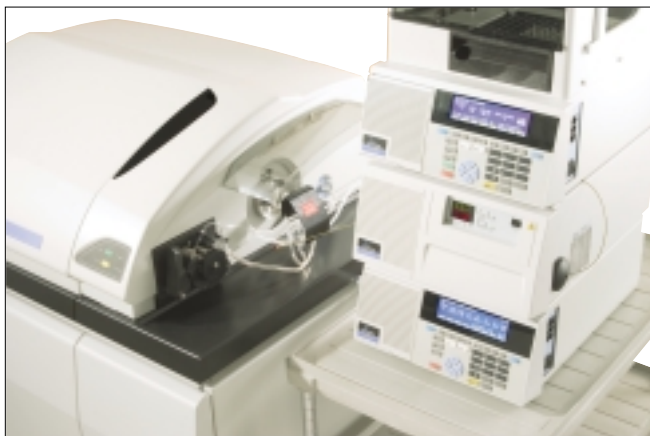
Figure 7. Chromatographic separations using the Series 200 HPLC system in conjunction with ICP-MS detection are used to perform speciation analysis.
