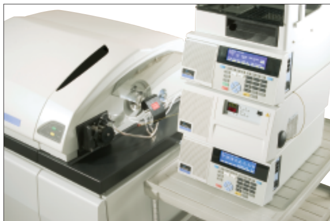
Figure 7. Speciation analysis is accomplished with the Series 200 HPLC system performing the separation and the ELAN providing detection.
