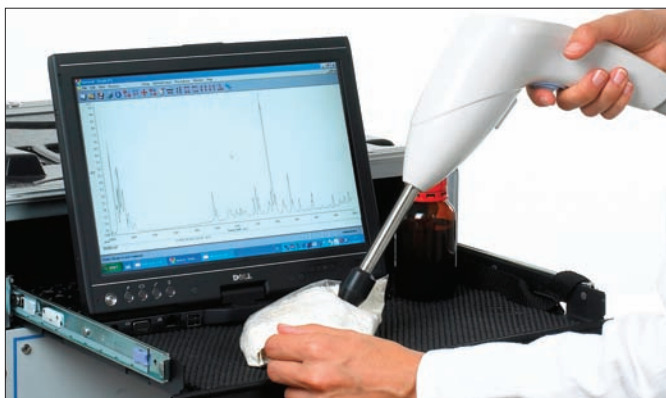
Figure 3. The hand-held trigger probe can be used for a range of samples.
